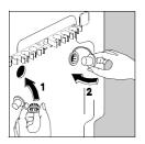
You can now see the openings that must be closed with the caches in the pack attached to the washing machine; do not forget to fold down the central capsule.
